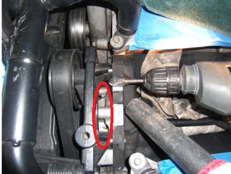
(Figure 4) I prefer a burr on a drill. Air tools work nice, but make a bigger mess.
